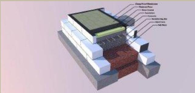
Solid concrete floors can have some benefits over a suspended floor because of low maintenance in the future and less prone to movement. They are normally up of different layers of materials which include:
