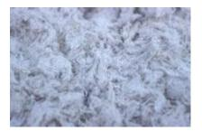
Loosely-bound asbestos materials are not commonly found in residential properties and were primarily used in commercial and industrial settings for fire proofing, sound proofing and insulation. In most cases, glass fibres have replaced asbestos in today's insulation products.
