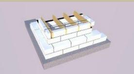
Suspended timber floors are normally made up of timber joists
