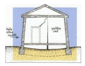
The dome effect causes the walls to tilt outwards and the restraining influence of the roof produces horizontal cracks on the outside wall. These will be wider on the outside surface rather than the inner.
