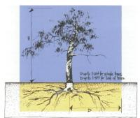
Diagram 3 on the next page shows the typical damage resulting from a large tree having been planted too close to the footings at a corner of a brick house – the tree has extracted the moisture from around and under the corner, resulting in subsidence. A tree root barrier would have restricted the spread of the roots and therefore the consequential water extraction form the soil under the footings.
